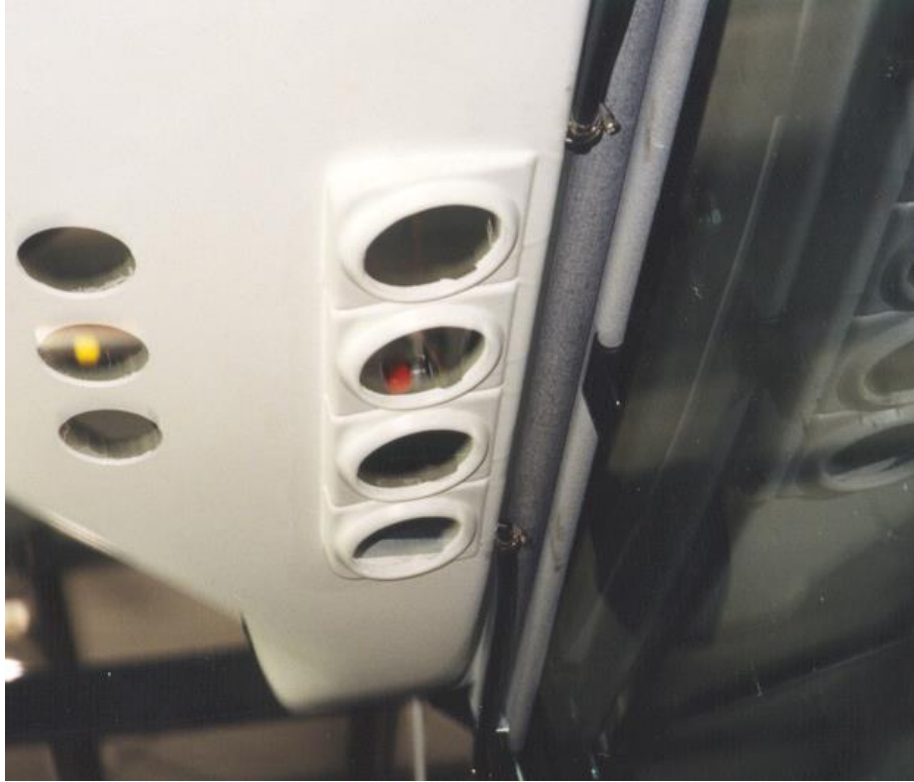
Drain tubes running along underside of headliner.
