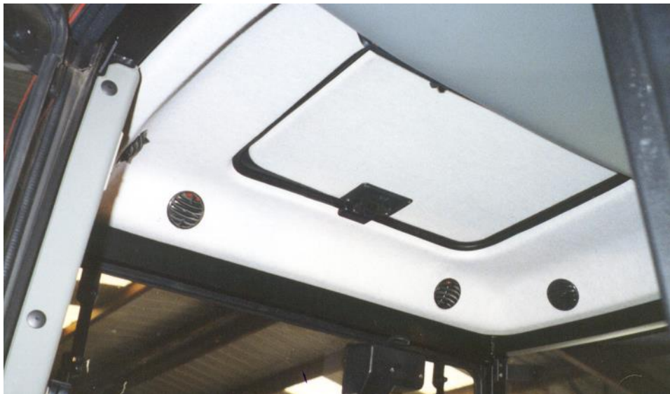
Rear recirculation louvers in place.
